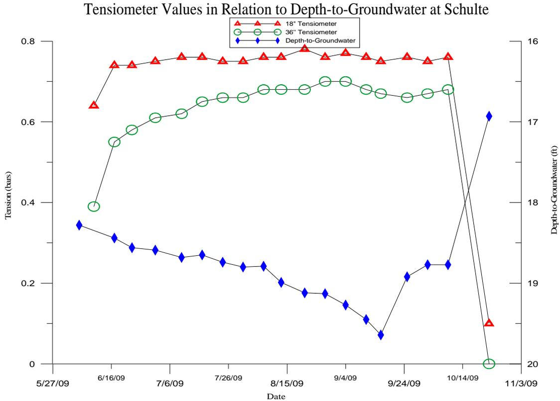
Figure 10: Schulte tensiometer soil moisture values vs. depth-to-groundwater at Reimers monitoring well.
