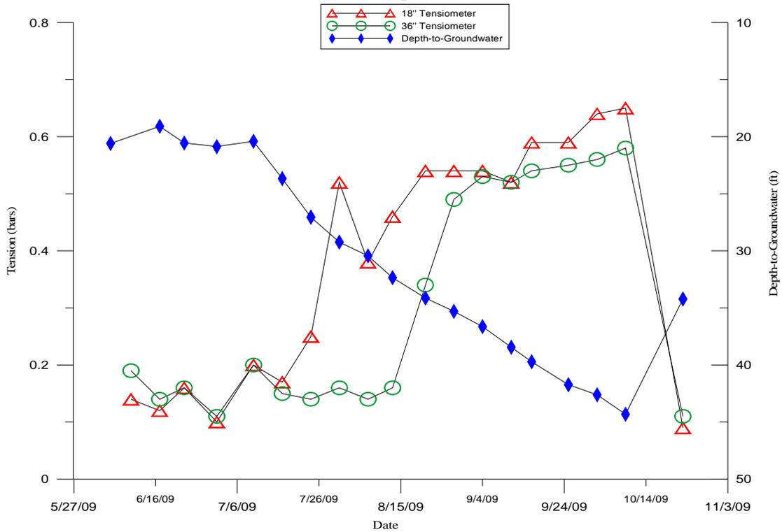
**Figure 7: Rancho Canada tensiometer soil moisture values vs. depth-to-groundwater at Canada East monitoring well.**
