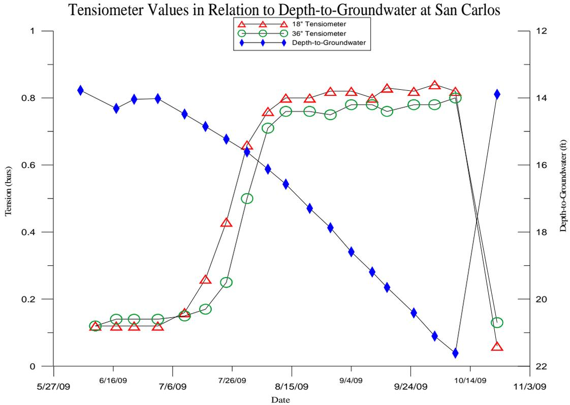
**Figure 8: San Carlos tensiometer soil moisture values vs. depth-to-groundwater at San Carlos monitoring well.**
