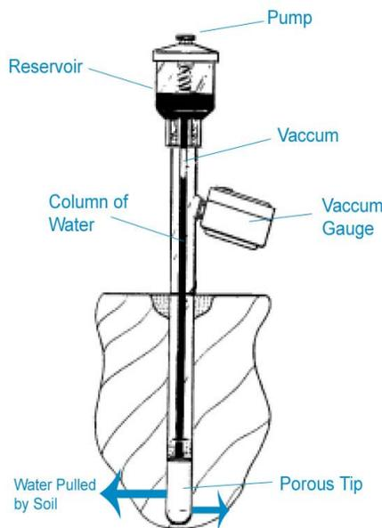
**Figure 2: A tensiometer consists of a sealed tube, a porous tip, a vacuum gauge, and a reservoir pump. The tube is buried with the porous tip at the bottom and water is hand-pumped into the tube from the reservoir. Once the column of water in the tube is filled, the device is left alone. Over time, the soil pulls the water out of the tube through a porous tip. A vacuum gauge then measures the attractive forces of the surrounding soil on the water filled column.**
