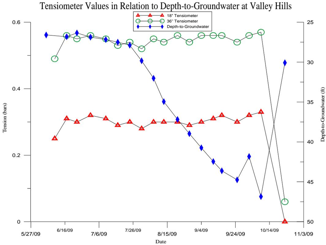
Figure 9: Valley Hills tensiometer soil moisture values vs. depth-to-groundwater at Williams South monitoring well.
